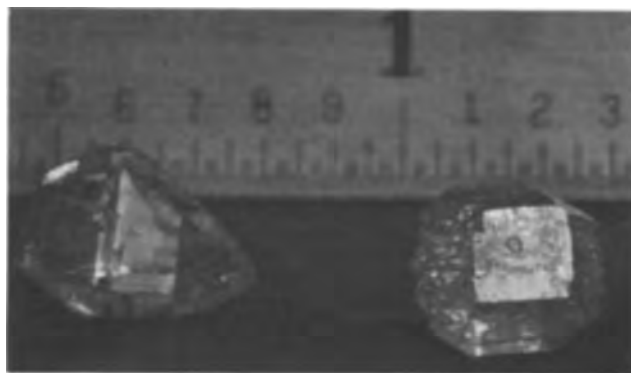
Fig. 3. BeO crystals grown from seeds shown in Fig. 1
