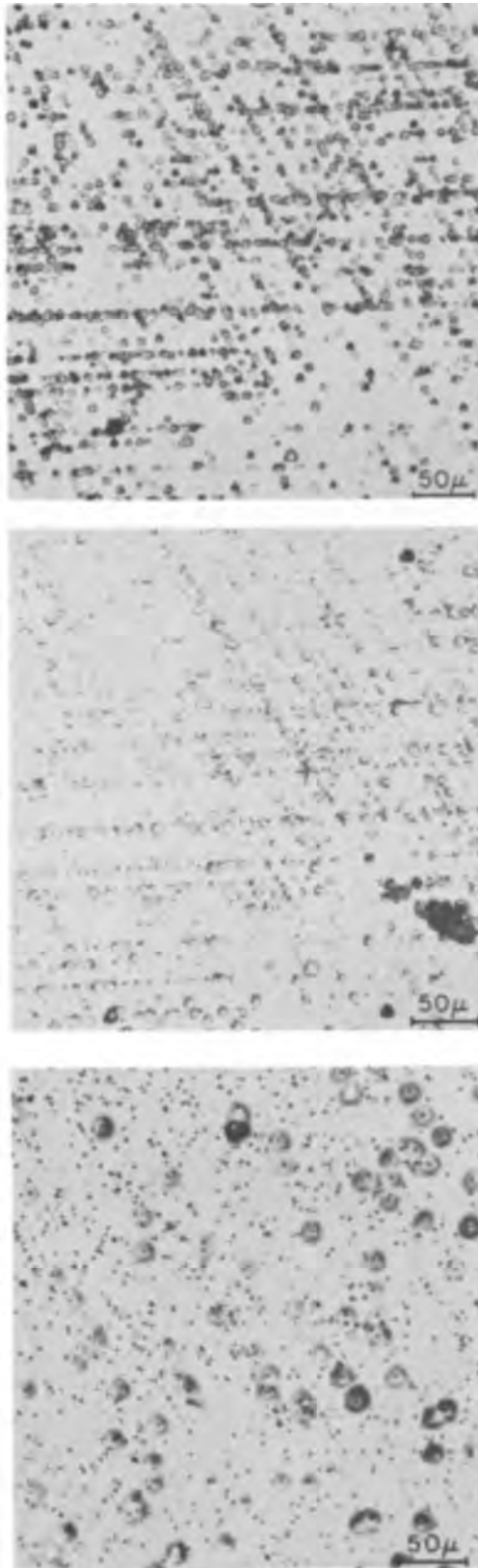
Fig. 9. Dislocation etch pits in a vapor-grown GaP crystal (a) (top); same area after 10\mu was removed by chemical polishing and followed by subsequent etching to reveal dislocations (b) (center); dislocation etch pits in a different area of the same crystal (c) (bottom).
