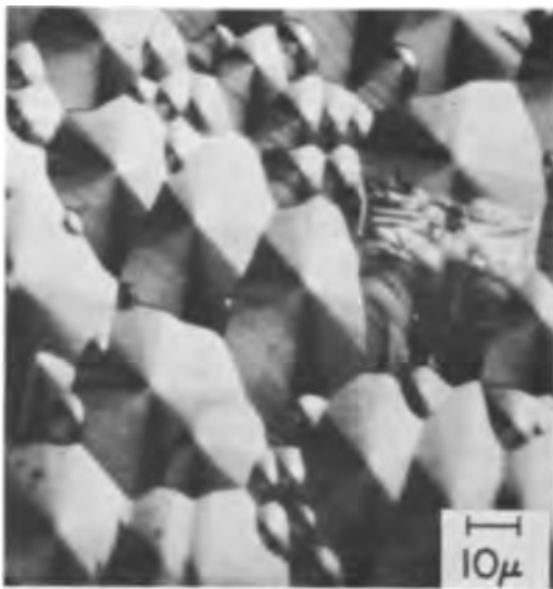
Fig. 5. Ge layer grown on semi-insulating GaAs at 600°C (thickness \sim 9\mu ).
