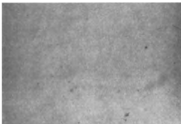
Fig. 1A. Reflection optical photomicrograph of laser evaporated film: germanium film on glass substrate. Magnification 350X.
