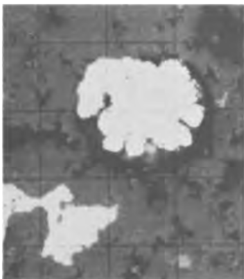
Fig. 7. Ag particles in an electrode discharged 65% at the 20-hr rate. Ag was the lightest shade in the photograph, \text{Ag}_2\text{O} dark gray, and the impregnation plastic was black. Small patches of \text{AgO} remaining in the \text{Ag}_2\text{O} are shown as a gray shade intermediate between Ag and \text{Ag}_2\text{O} . Compare Ag particle newly formed by electrolytic reduction (upper) with Ag particle that had not oxidized completely in the previous charge (lower left). Original magnification 1600X.
