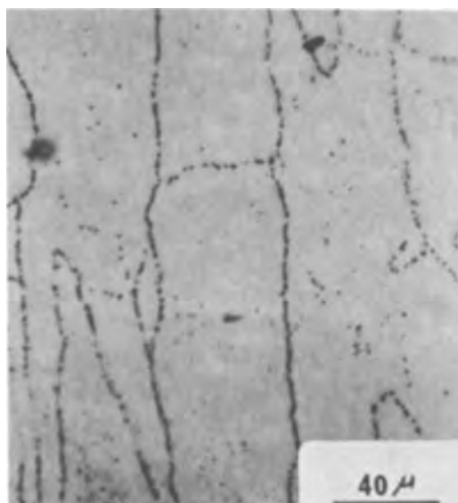
Fig. 5. Columnar subgrains in crystal annealed for 5 hr at 1100°C
