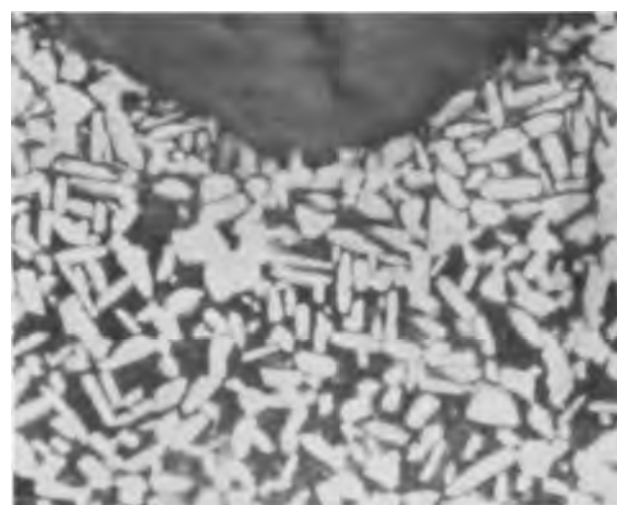
Fig. 4. Alloy microstructure beneath oxide scale in specimen oxidized at 870°C (400X).
