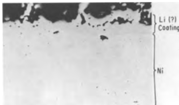
Fig. 5. Photomicrograph of a (10:1 taper section) nickel sample which was run at 900^\circ\text{C} for 6 hr. Magnification ca. 200X.
