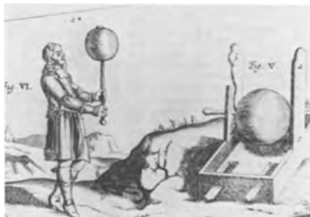
Fig. 3. Von Guericke's frictional electrostatic machine is on the right. On the left, the burgomeister is demonstrating how a feather a , first charged by contact with the sphere, may be made to move about in the air as he chose. This is probably the earliest example of achieving the directed motion of a particle under the action of an electric field (7).
