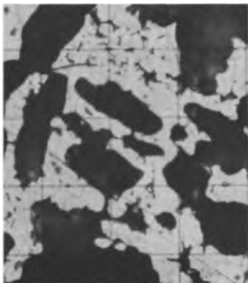
Fig. 11. Coarse dendritic crystals of Ag present in some areas of the discharged electrode of Fig. 9. Angles of approximately 90 degrees were often present. Compare with Fig. 8 and 10 at the same magnification.
