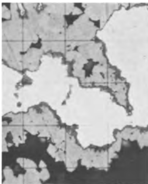
Fig. 15. Electrode appearance after oxygen evolution began at end of sixth charge. The large Ag particles that had formed during slow discharges did not oxidize as extensively as the small Ag particles originally present. Compare with Fig. 14 at the same magnification.
