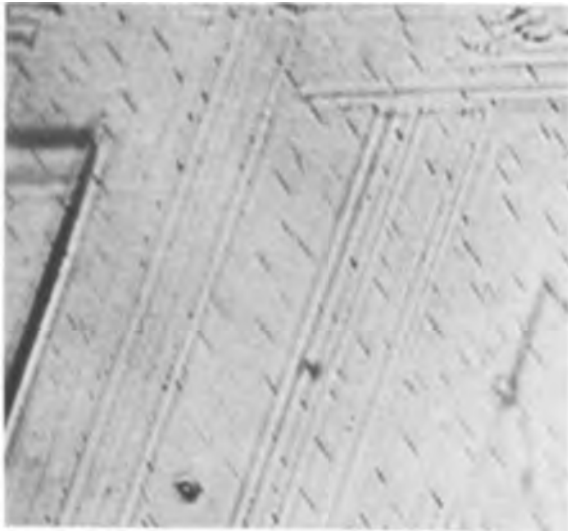
Fig. 4. Sequence of hot stage photomicrographs showing the growth and dissolution of thermal facets as a function of oxygen partial pressure at 1000°C. Optical micrograph. Fig. 4a, 3 min at 1.2 \times 10^{-5} Torr. Magnification ca. 700X.
