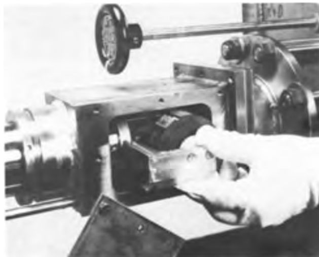
Fig. 2. Receiver design showing vacuum port for loading sample holder.
