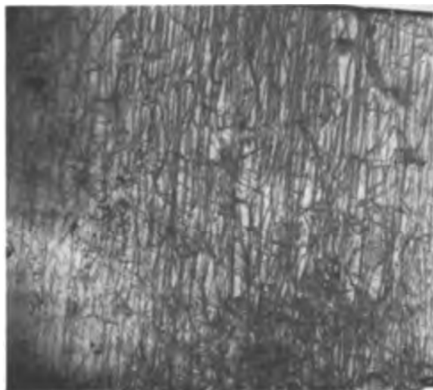
Fig. 4. X-ray topograph of a gallium antimonide wafer exhibiting a high density of dislocations. Two sets of dislocations can be observed. One set of rather long dislocations appears aligned along the \langle 111 \rangle growth direction, the other consists of a network of dislocation loops. Ag, K\alpha radiation (220) reflection. Magnification ca. 40X.
