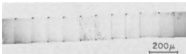
Fig. 8. Etched angle-lapped surface of a GaP crystal (left) grown by vapor deposition on a nearly dislocation-free GaP substrate (right). The high density of etch pits is coincident with the substrate-growth interface.
