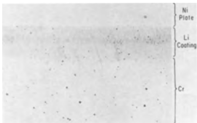
Fig. 1. Photomicrograph of a transverse cross section of a chromium sample run at 900°C in LiF for 10 min. Tapered section, \sim 8:1 . Magnification ca. 100X.
