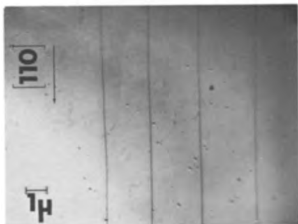
Fig. 4. SOT x-ray topograph of diffused structures similar to Fig. 3 with the following thicknesses of surface removed: a, nothing removed; b, 0.5\mu ; c, 10.0\mu ; d, 19.0\mu .
