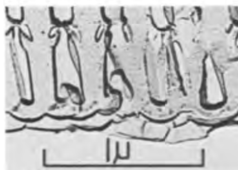
Fig. 3. Electron micrographs of sections through anodic films formed in 4% w/v phosphoric acid (a, top) 10 min after changing from 87 to 117.5v, showing pore joining and termination; (b, bottom) 13 min after changing from 117.5 to 87v, showing pore branching and incipient pore formation.
