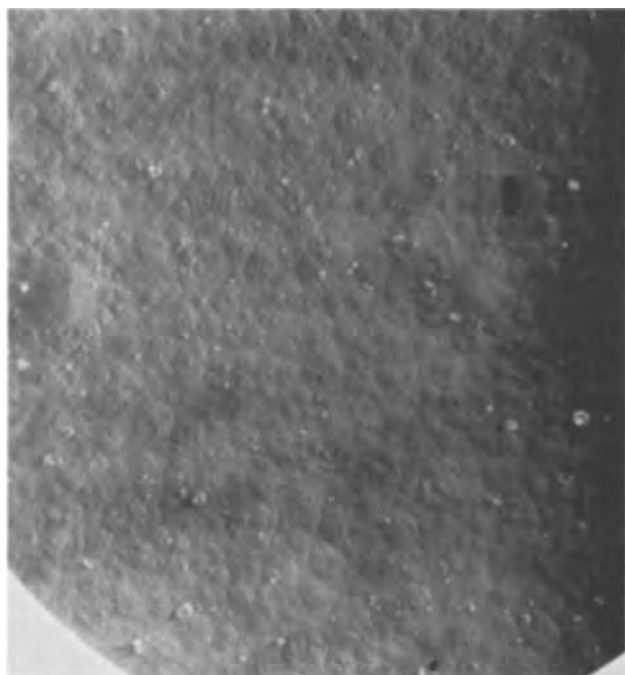
Fig. 4. Electron micrograph of a V_2O_5 film on sapphire at ca. 7600X.
