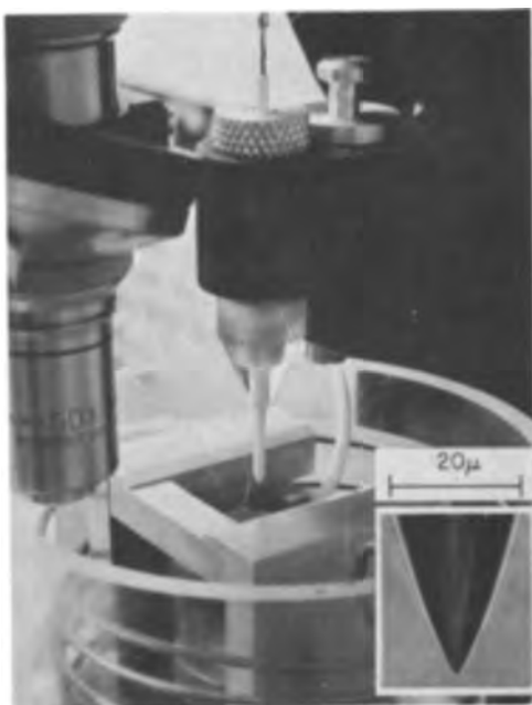
Fig. 1. Experimental arrangement showing microprobe, specimen, thermocouple, and specimen heating bath. Insert shows profile of mechanically polished probe tip.
