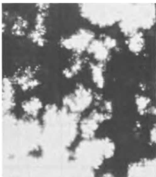
Fig. 13. \text{Ag}_2\text{O} that formed on Ag during sixth charge when electrode was charged to the potential peak that begins \text{Ag}_2\text{O}/\text{AgO} potential plateau. Compare with Fig. 12 at the same magnification.
