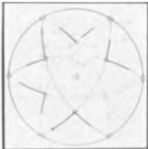
Fig. 6. The location of observed facets on the tip of molybdenum dendrites shown on a stereograph projection in the growth direction. Heavy lines indicate location of optical reflections along 100 zones.
