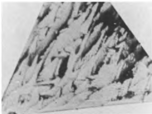
Fig. 2. Photomicrograph taken with transmitted light of \langle 111 \rangle surface of epitaxially-grown GaP. Magnification ca. 18X.
