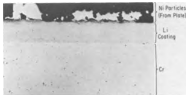
Fig. 3. Photomicrograph of a transverse cross section of a chromium sample run at 1000°C in LiF for 30 min. Tapered section, \sim 10:1 . Magnification ca. 50X.
