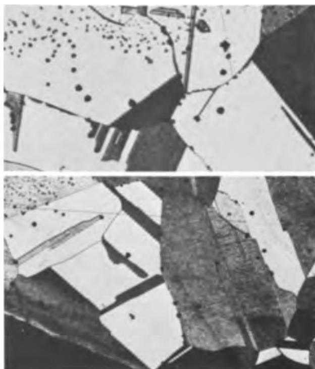
Fig. 1. Nucleation of silver at high angle grain and twin boundaries. The nuclei appear as black spots. Fig. 1a (top) Cell voltage 25mv, average current density 1 ma/cm 2 , etched. Magnification ca. 30X. Fig. 1b (below) Cell voltage 25 mv, average current density 1 ma/cm 2 , etched. Magnification ca. 28X.
