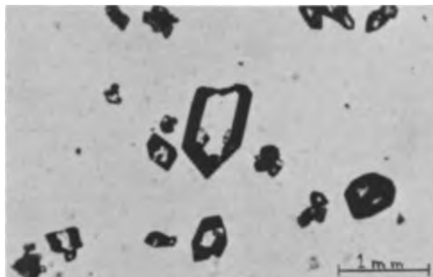
Fig. 1. Photomicrograph of hydrothermally grown single domain \text{LiNbO}_3 crystals.
