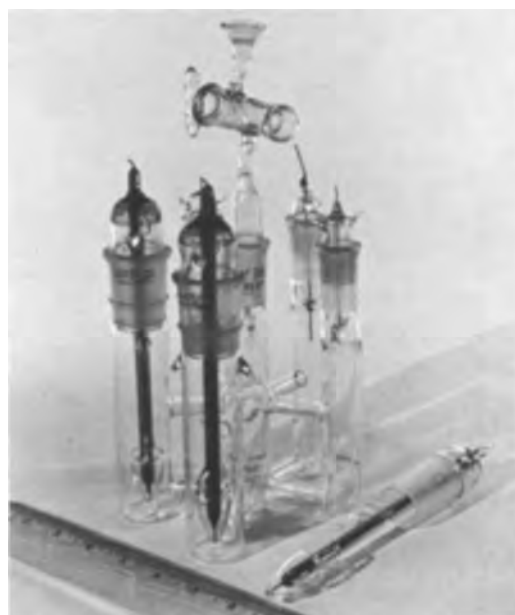
Fig. 1. Five-compartment cell used for emf measurements
