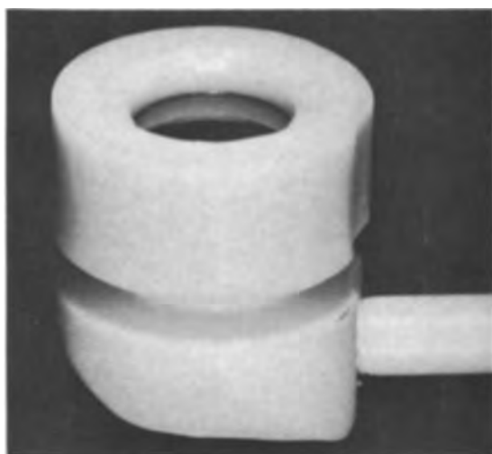
Fig. 1. GaAs wafer in a Teflon holder (electrode)
