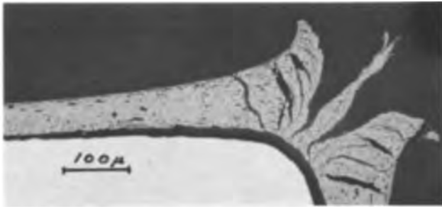
Fig. 6. Cross section of specimen oxidized at 380 Torr, 575°C for 32.5 min, showing normal edge effect. Magnification 125X.
