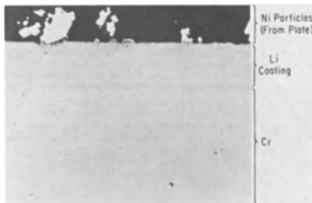
Fig. 4. Photomicrograph of a transverse cross section of a chromium sample run at 1000°C in LiF for 120 min. Tapered section, \sim 10:1 . Magnification ca. 50X.
