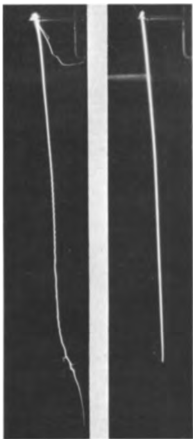
Fig. 1. Time-exposed track photographs of 377\mu -diameter aluminum droplets as they burned in free fall (a, left) in air and (b, right) in a mixture of 20% oxygen in argon, with total gas pressures in both cases at 625 Torr. Short traces emanating from holder arise from tiny droplets formed from crossed aluminum fiber support. Note the typical erratic trace that appears when an aluminum droplet burns in air.
