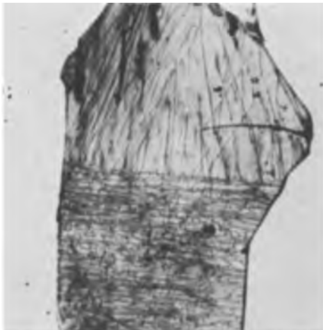
Fig. 2. X-ray topograph of partially regrown gallium antimonide wafer. The regrown region exhibits a marked decrease in the dislocation density; Ag, K\alpha radiation; (220) reflection. Magnification ca. 20X.
