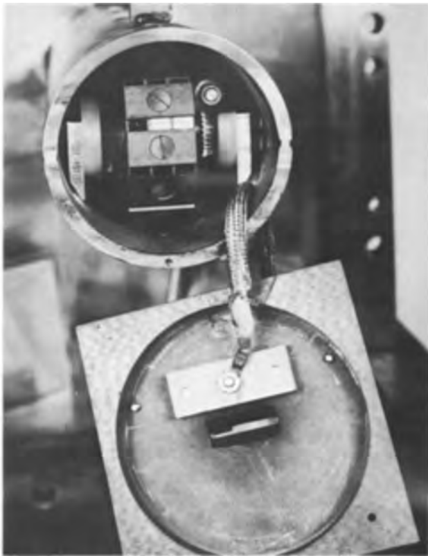
Fig. 3. Receiver design showing sample positioning in beam
