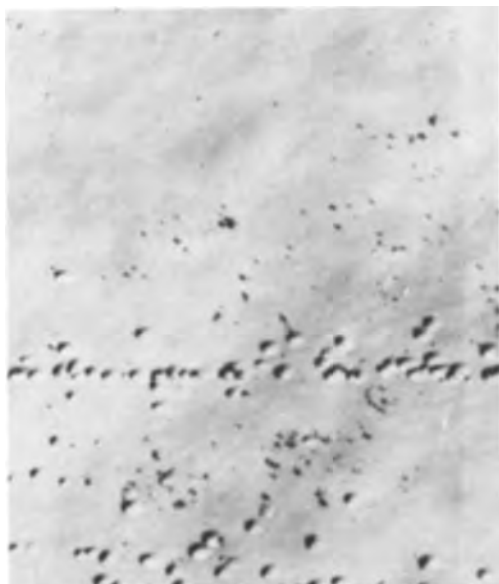
Fig. 4a. Photomicrograph of alloy heterojunctions, \text{Ga}_{0.9965}\text{In}_{0.0035}\text{Sb} on GaSb. Magnification 300X.
