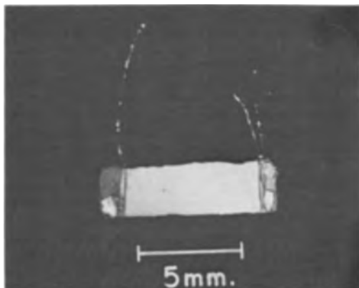
Fig. 2. Specimen of \gamma\text{-Nb}_2\text{O}_5 stripped from a niobium specimen oxidized at 760^\circ in 1 atm oxygen for 120 min.
