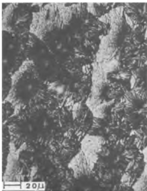
Fig. 1. Photomicrograph of the surface of a nitrided silicon wafer. Magnification ca. 330X.
