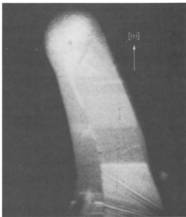
Fig. 6. Curved silicon crystal photographed during nonisothermal growth. Magnification approximately 50X.
