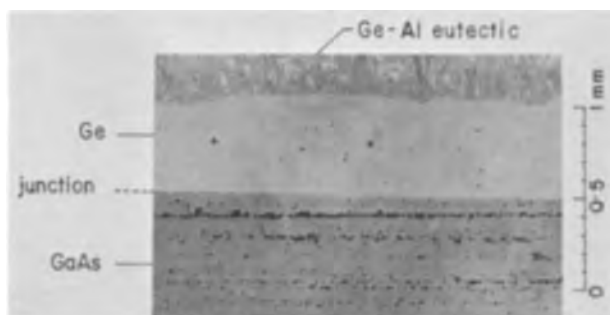
Fig. 10. Polished cross section of the Ge-GaAs junction fabricated by crystallization of Ge from the Al-Ge alloy solution. (Higher magnification).
