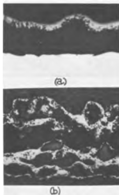
Fig. 4. Cross sections of scales on Fe-59.5% Cr: (a) 5 hr at 1000°C, magnification ca. 500X; (b) 5 hr at 1200°C, magnification ca. 250X.
