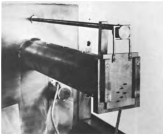
Fig. 4. Receiver design showing beam current monitoring technique.
